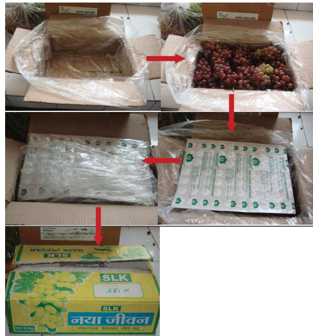
Figure 3: Packaging in corrugated fibre board boxes with polyethylene liner and a grape guard
