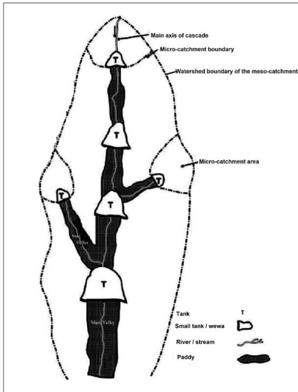
**Figure 1:** Schematic diagram of a tank cascade system (Panabokke *et al.*, 2002)
